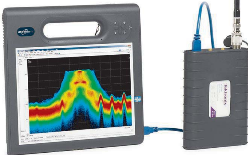
1. Tektronix's RSA3360 6-GHz spectrum analyzer, coupled with a PC or tablet running the company's freeware, facilitate frequency-domain analysis in the field, on the benchtop, or in the university classroom or lab.
