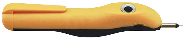
3. Costing roughly $100, the 25-MHz digital oscilloscope-in-a-pen connects to a PC via USB. It handles input-signal amplitudes ranging from 5 to 50 V.
