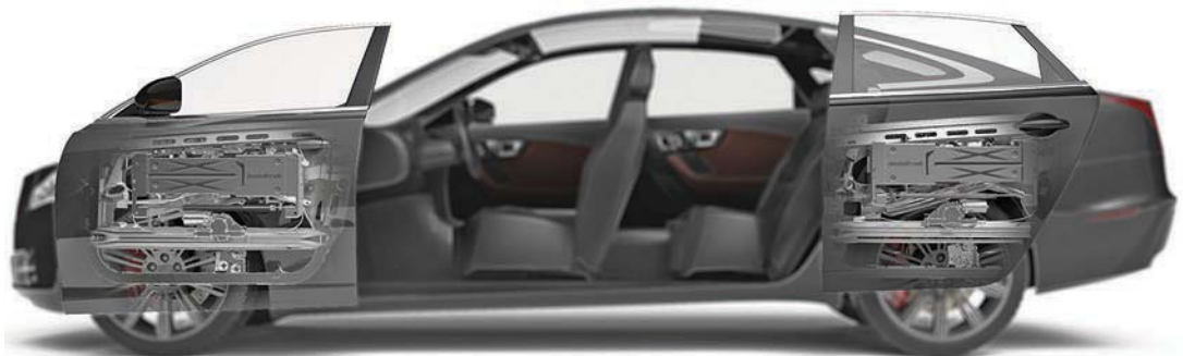
Dura Automotive Systems used Dassault Systems' Solidworks design tools and the Simulia simulation system to design and simulate the sliding French doors including the mechanical, electrical, and software environment.
