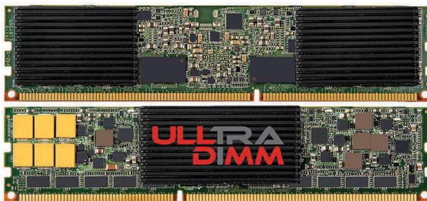
1. SanDisk UltraDIMM (top/rear, bottom/front) plugs into a standard DDR DIMM socket but it contains flash memory. It can be updated at the row level instead of the block level required for disk storage.
