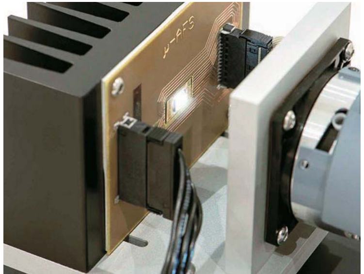
A research team has developed an LED chip with an array of 256 pixels as part of a project to develop more advanced LED headlamps. (Image courtesy of Osram Opto Semiconductors)
